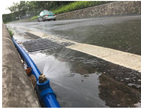
The working water drenching instruments in South China University of Technology, Guangzhou, China
